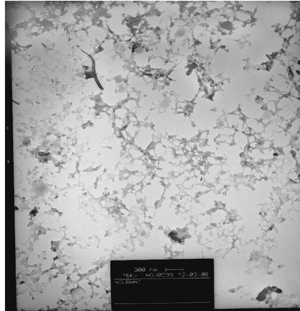
Fig. 1 – Transmission Electron Microscopy of PMMA/CNT nanocomposites
